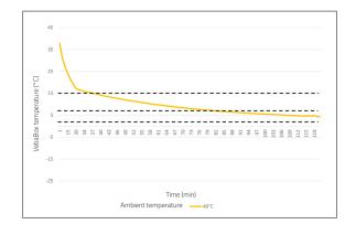
Heating performance at ambient temperature Model Q Cool
